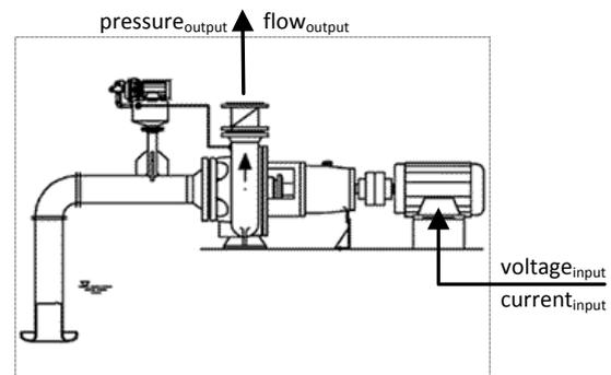
**Fig. 7: Each device has input and output pairs of effort and flow variables.**
