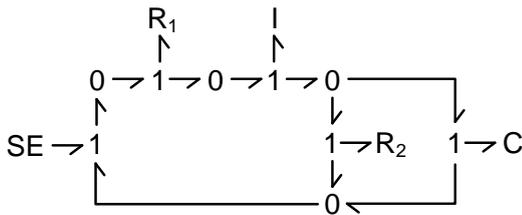
**Fig. 9: Bond graph for the electrical circuit, incl. components, junctions, and directed power flows and voltage ( $v$ ) as output, or vice-versa.**
