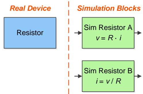
**Fig. 10: Problem of 1:n mapping between real devices and simulation blocks. For example, a real device resistor can be simulated by either a resistor approximation having electrical current ( $i$ ) as input.**
