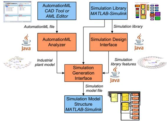
**Figure 6: Proposed method for simulation model generation.**
