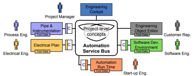
The **parallel engineering of industrial plants** demands the effective and efficient collaboration of domain experts, such as mechanical, electrical, and software engineers, and of their specialized software tools. While there are attempts to impose fixed sets of software tools, which work well together, the reality in most projects is a “best of breed” collection of software tools that were not designed to cooperate seamlessly.
